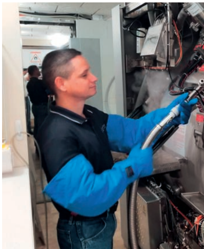
Above and above right: Liquid helium is used to keep the superconducting magnets cool in an MRI machine. The same concept is utilised in the Large Hadron Collider to accelerate particles to near the speed of light.
